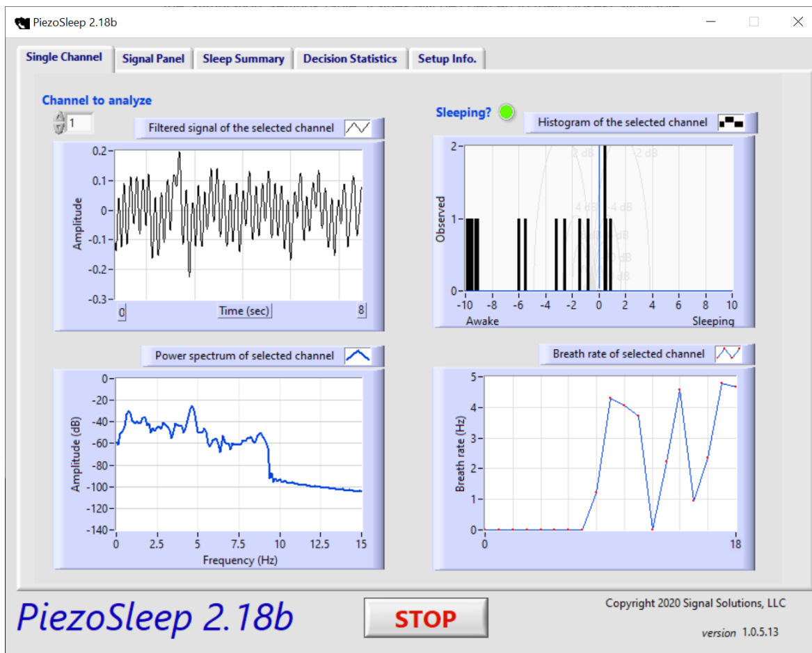
Figure 8. Single Channel tab showing the recorded signal (top left), sleep decision statistic (top right), power spectrum (bottom left), and the breath rate frequency (bottom right) for an individual channel.
